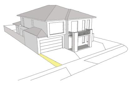
It is recommended that homeowners install a 100mm diameter PVC conduit under the driveway to accommodate any future irrigation requirements for the planting strip.
